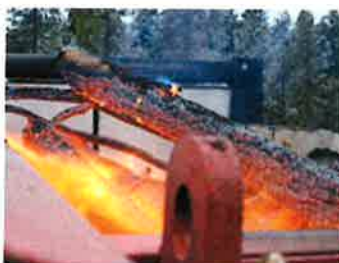
Figure 5— Photo shows results when the airflow is broken; a log smolders above the air curtain.
