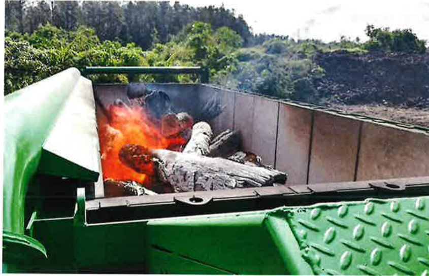
FireBox in Operation: Particulate Matter (PM) trapped by Air Curtain and re-burned
