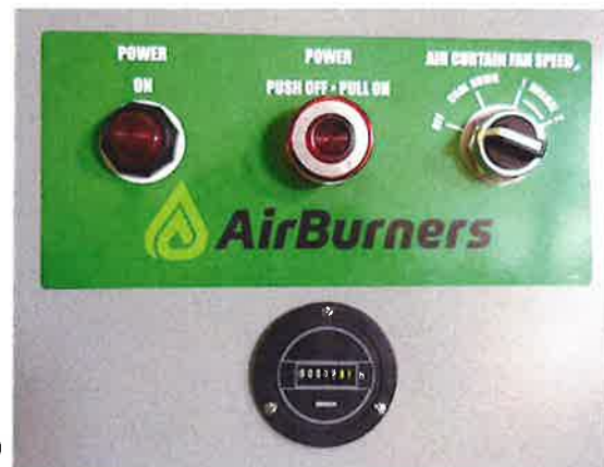
Control Switches, Indicator Lights & Hour Meter
